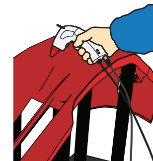
Dust and static-electricity removal from bumpers
