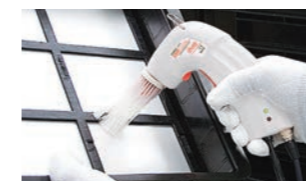
Attach a brush to blow out dust
